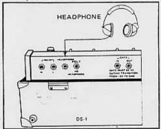
A toggle switch on the front panel designates whether the signal from the synthesizer will go to the head phones or the amplifier.
