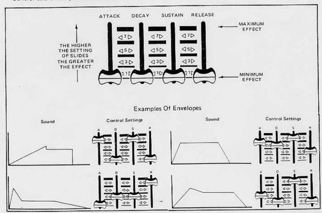
If you stop playing a note before the sustain level has been reached, the envelope will go from where it was left off to 0 at a pace determined by the Release Control.
