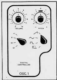
The Oscillator 1 generates the source or raw sound which will be modified by the other controls on the synthesizer. This is your primary oscillator so use it to tune to a-440 or to the other instruments in the group.
