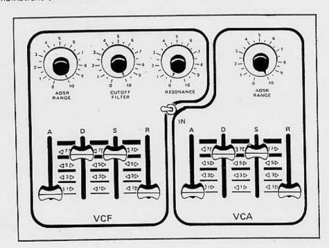
This ADSR works the same as the filter ADSR, and the ADSR Range Control again determines the amount of effect the ADSR has on the VCA. By throwing the toggle switch in-between the the VCF (Voltage Controlled Filter) and the VCA to the left, the Filter's ADSR operates both the VCF and the VCA. This can be used for quick set-ups and changes in live performances.
