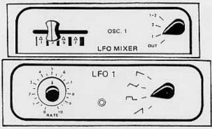
Turn off the volume of OSC.2, Noise, and Poly so as to more clearly hear what is happening. Now the frequency of OSC.1 will vary depending on the speed of LFO 1 (.3 Hz to 30 Hz) and the amount of modulation allowed in at the mixing bank. Play around with these controls as well as the wave shape of LFO 1 until you are familiar with how it affects the sound.
